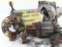
Unit has been run in mesh and has literally exploded due to running at engine speed. The centrifugal force has simply blown the starter apart.
