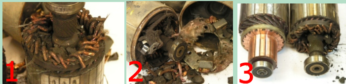
Pictures 1 & 2 show the effects of a starter "running in mesh". Picture 3 shows a "before and after" armature. The "after" has clearly exploded.
